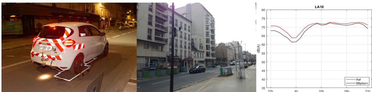
Figure 4: CPX measuring equipment (City of Paris); Acoustic station and thermal station; Frémicourt street 75015 Paris (SMaphon); LA10 indicator (Courcelles street).
